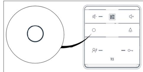
If the LED of the speech button lights up **green**, the Smart Stick **can be used** in the indoor station.
