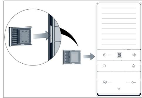
The ambient lighting briefly lights up green. The Smart Stick PHONE has been recognised. The Smart Stick PHONE automatically goes into configuration mode. The ambient lighting flashes orange.
