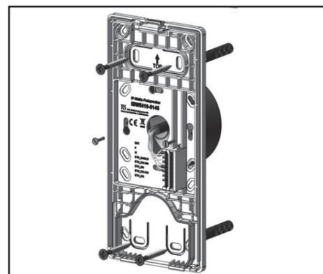
Guide the connection cable through the cable gland. Connect the wires to the terminal according to the labeling
