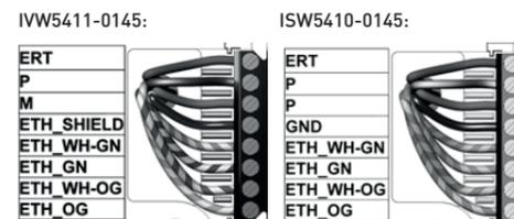
**CAUTION!** Device damage due to interchanging the connections between ISW5410 and IVW5411.
